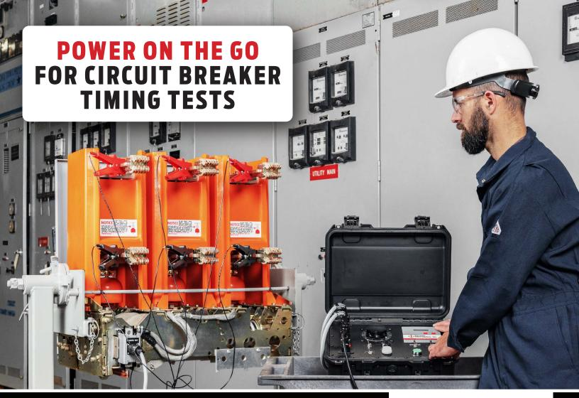
CBT-1202 includes heavy-duty circuit breaker timing test set, variable power supply, and switching controls in one unit.
