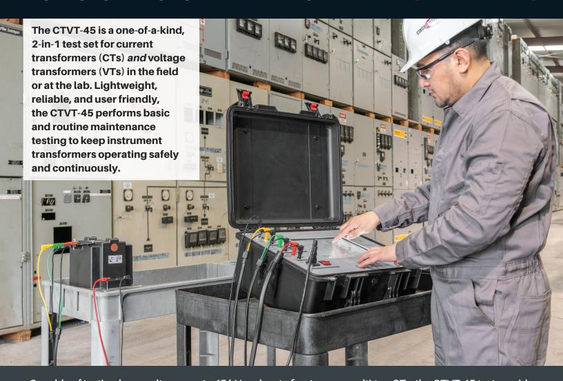
Capable of testing knee voltages up to 45 kV and up to five taps on multi-tap CTs, the CTVT-45 tests a wide range of instrument transformers, including those in protection and metering applications. The device combines all-in-one testing with high accuracy and resolution to provide reliable and efficient equipment maintenance. The CTVT-45 can also store up to 5,000 data files to help keep maintenance reports accurate.
