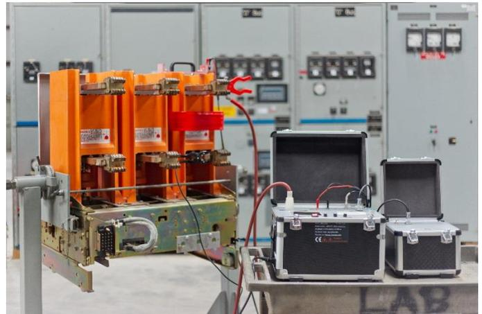
Figure 9. Rigid, magnetic coil applied to an entire pole
