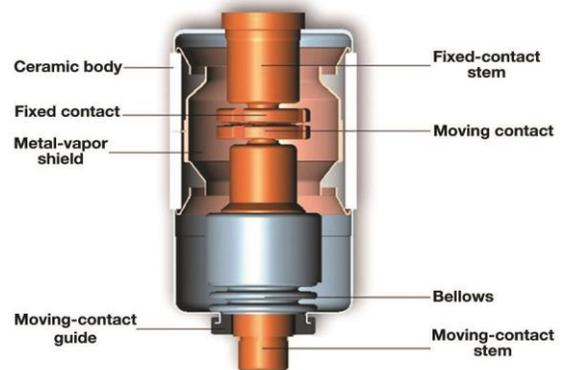
Figure 2. Internal view of a typical vacuum interrupter
