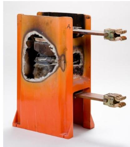
Figure 5. Failed vacuum interrupter
